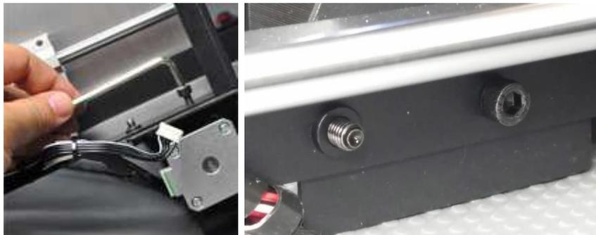
9. Use a carpenter's level to ensure that your flat surface is level. If it is not level, locate a level surface and place the printer on top of it. Next use the carpenter's level to check that the X-axis guide rods are level. If not, raise or lower either side by manually turning the Z-axis couplers on either side of the frame.
