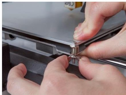
21. Now that the printer is off you can manually move the extruder around the build platform. Because most printing is done near the center of the platform, you should check the nozzle height at points about 2 inches from each corner, as indicated by the blue X marks in the diagram below.
