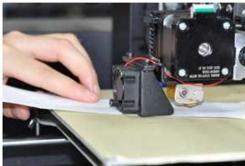
22. Switch the printer on and wait for it to initialize. Select **Position > Z. Pos. Fast**, then turn the knob to raise the extruder so that it is at least an inch above the build plate.
