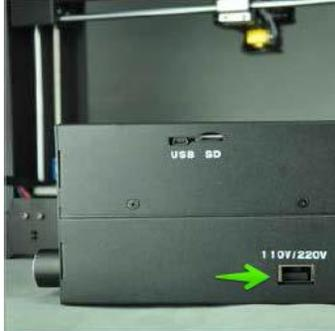
18. Ensure that the power switch is in the OFF position (O side depressed). Plug the C13 end of the included **AC Power Cable** into the C14 panel connector on the **Power Supply/Control Box**, then plug the other end into a nearby AC power outlet. Depress the I side of the power switch to power the printer ON.
