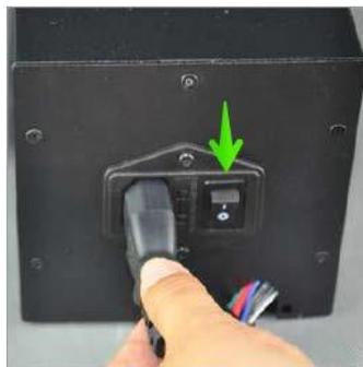
19. Wait for the printer to warm up and initialize. When it is ready, it will display *Printer ready* at the bottom of the LCD display. Select **Quick Settings > Home All**. Wait for the printer to move the build platform and extruder to the home position, then turn the printer off.
