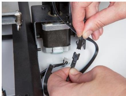
14. Insert the white connector on the shortest of the three cables into the corresponding white connector on the left side Z-axis stepper motor.
