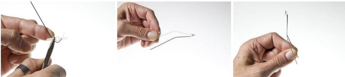
Put the two ends of the wire leg through the second hole from the center and then bend the two legs apart, as seen in the images above. Hold the wire leg and the servo horn with pliers and bend the wire down close to the servo horn.
