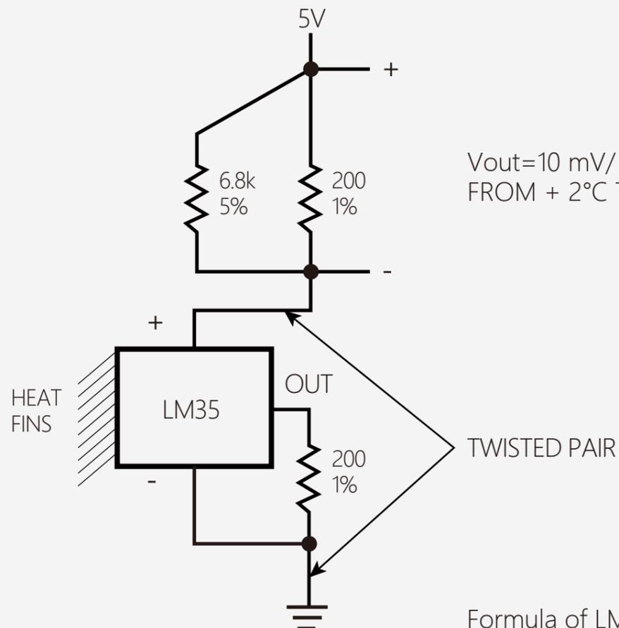
$$V_{out} = 10 \text{ mV}/^{\circ}\text{C} (\text{TAMBIENT} + 1^{\circ}\text{C})$$
