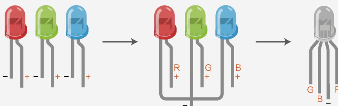
Fig. 5-2 How 3 LEDs form A RGB LED (Common Cathode)
