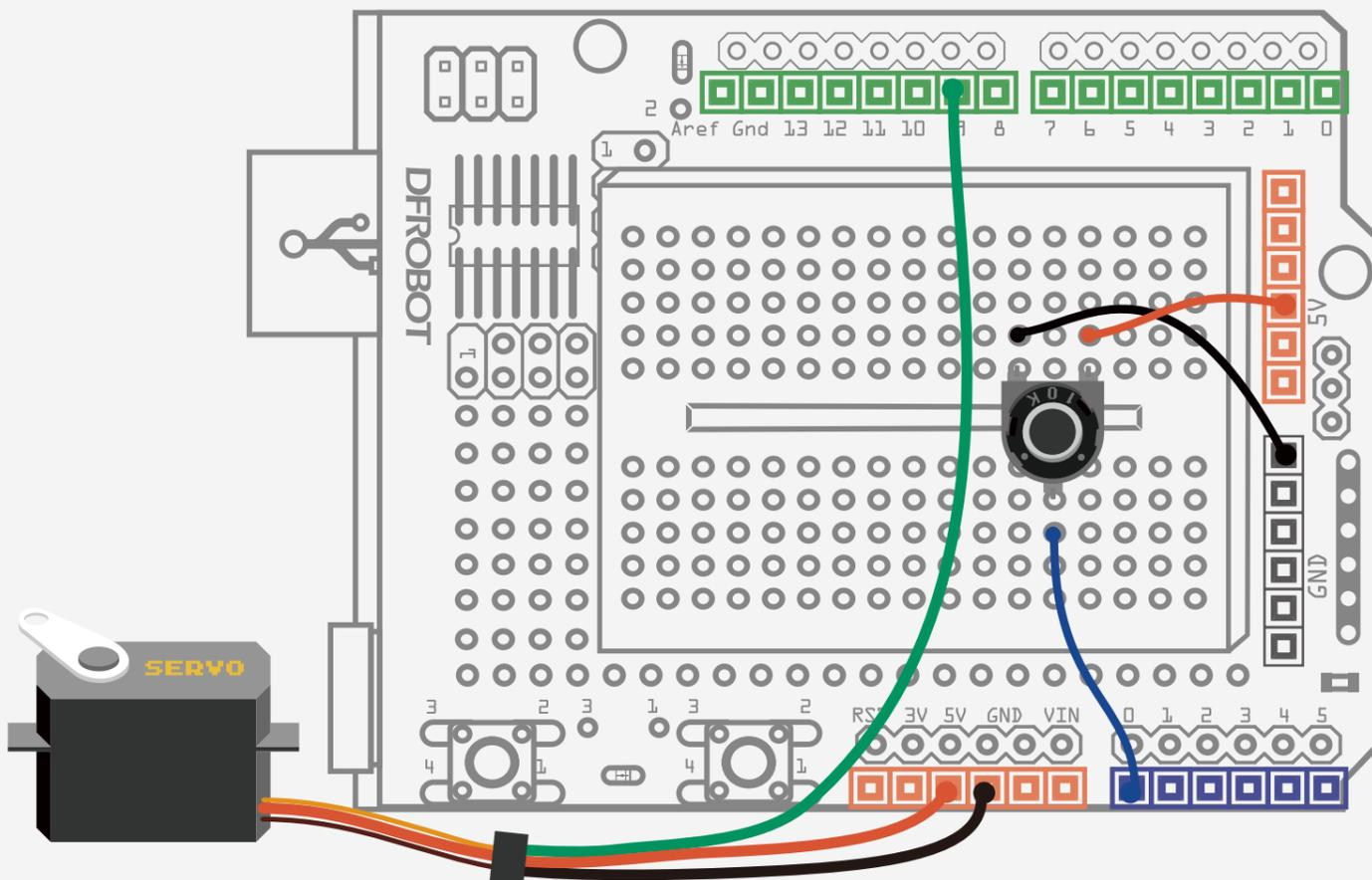
Fig. 11-1 Controllable Servo Circuit Diagram
