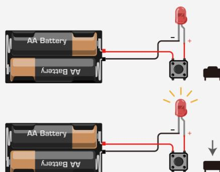
Fig 3-4 button diagram
