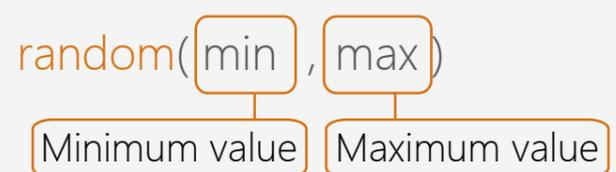
The first variable of this function is the minimum value and the second is the maximum. So we configure as "random(0,255)" in this program.
