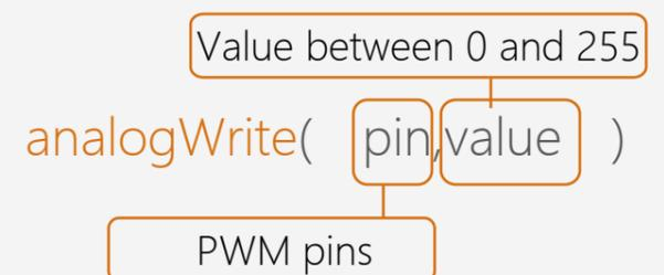
The `analogWrite()` function is to assign PWM pin an analog value between 0 and 255. Beware that `analogWrite()` can also used for PWM pins.
