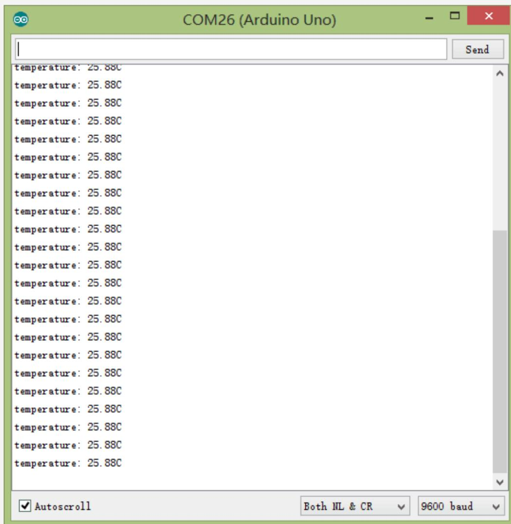
As per the program, once the temperature reaches 27 degrees C, the buzzer starts to sound. If the temperature drops below 27 degrees C, the buzzer stops.
