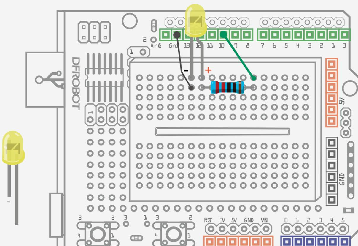
Fig 1-1 LED Flashing Circuit
