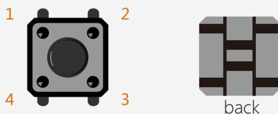
Fig 3-2 Structure of push button (front & back)
