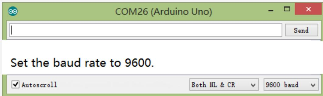
Read temperature value from the serial port. If you put your fingers on the LM35 sensor, you will find the temperature rises immediately. Your fingers are transferring heat to the sensor!
