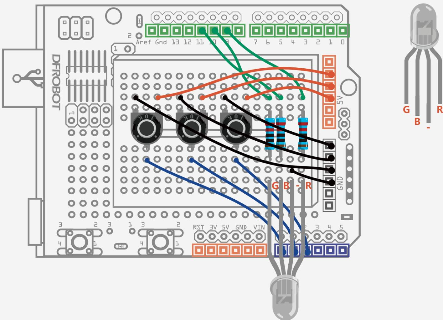
Fig. 12-1 Interactive Adjustable RGB LED Circuit diagram
