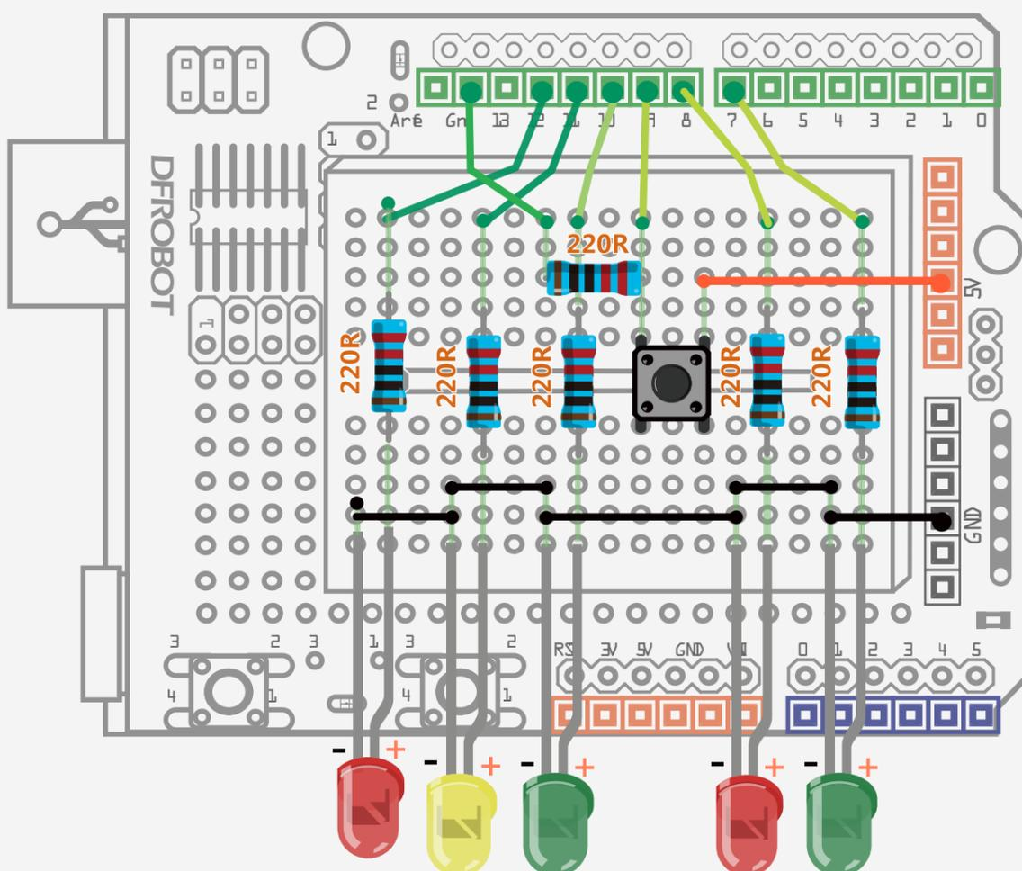
Fig 3-1 Wiring Diagram of LED Blinking
