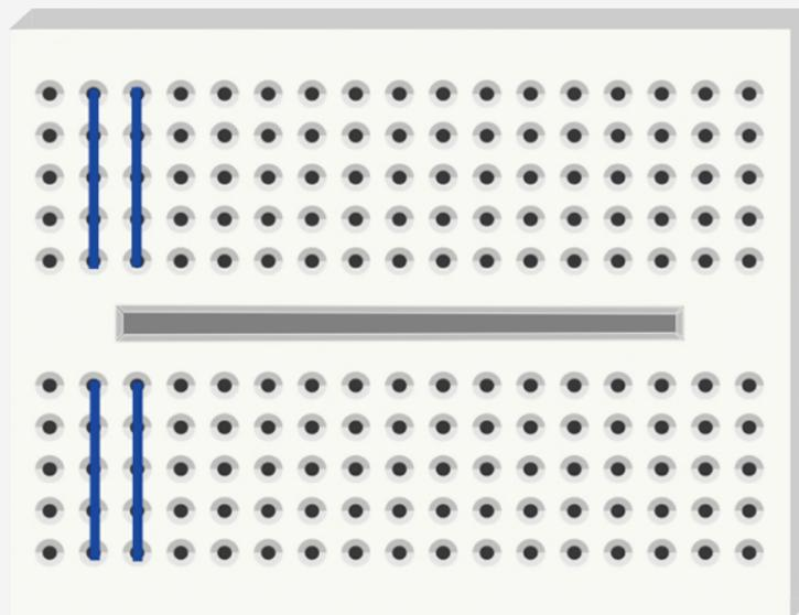
Fig 1-2 Breadboard Conductivity Direction
