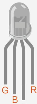
Fig. 5-4 Common Cathode RGB Diagram
