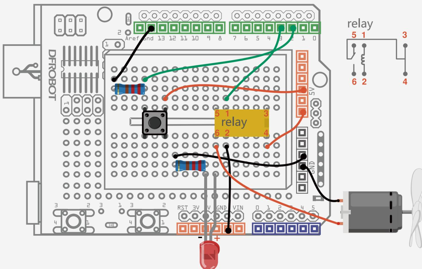
Fig. 13-1 DIY Fan Circuit Diagram
