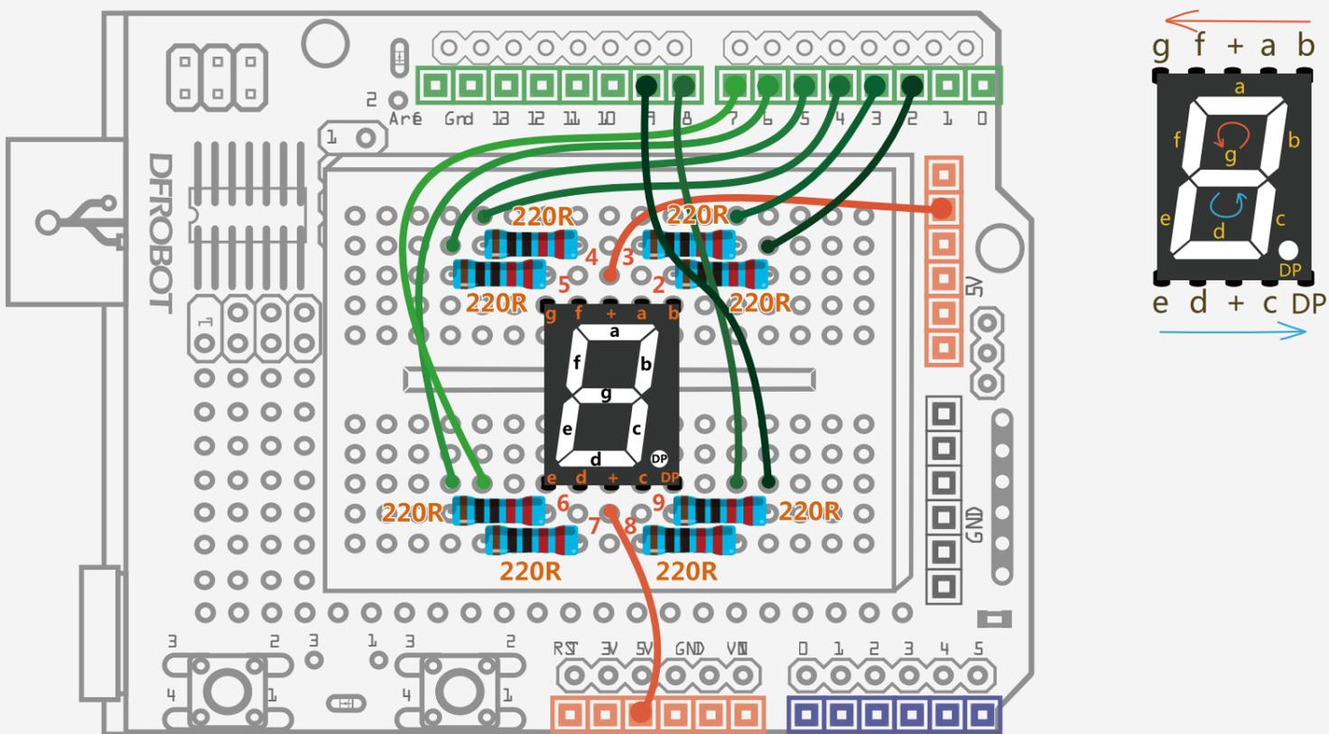
Fig. 15-1 LED Module Display Circuit Diagram
