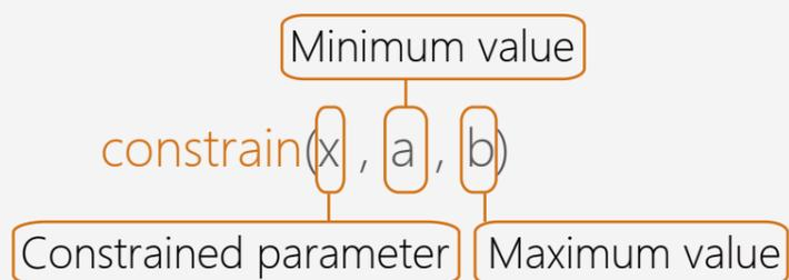
The "constrain()" function requires three parameters: x, a and b.
