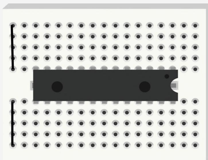
Fig 1-3 DIP Chip Inserted
