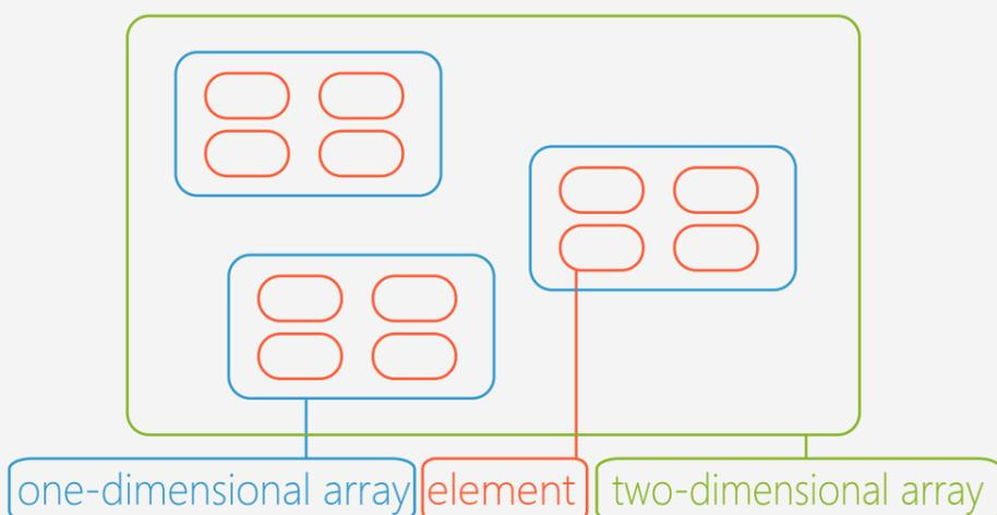
In the first sketch, we manipulated 10 arrays, each with 8 elements corresponding to values in the segment from b to DP. In this sketch, we will manipulate 10 one-dimensional arrays together to form a two-dimensional array.
