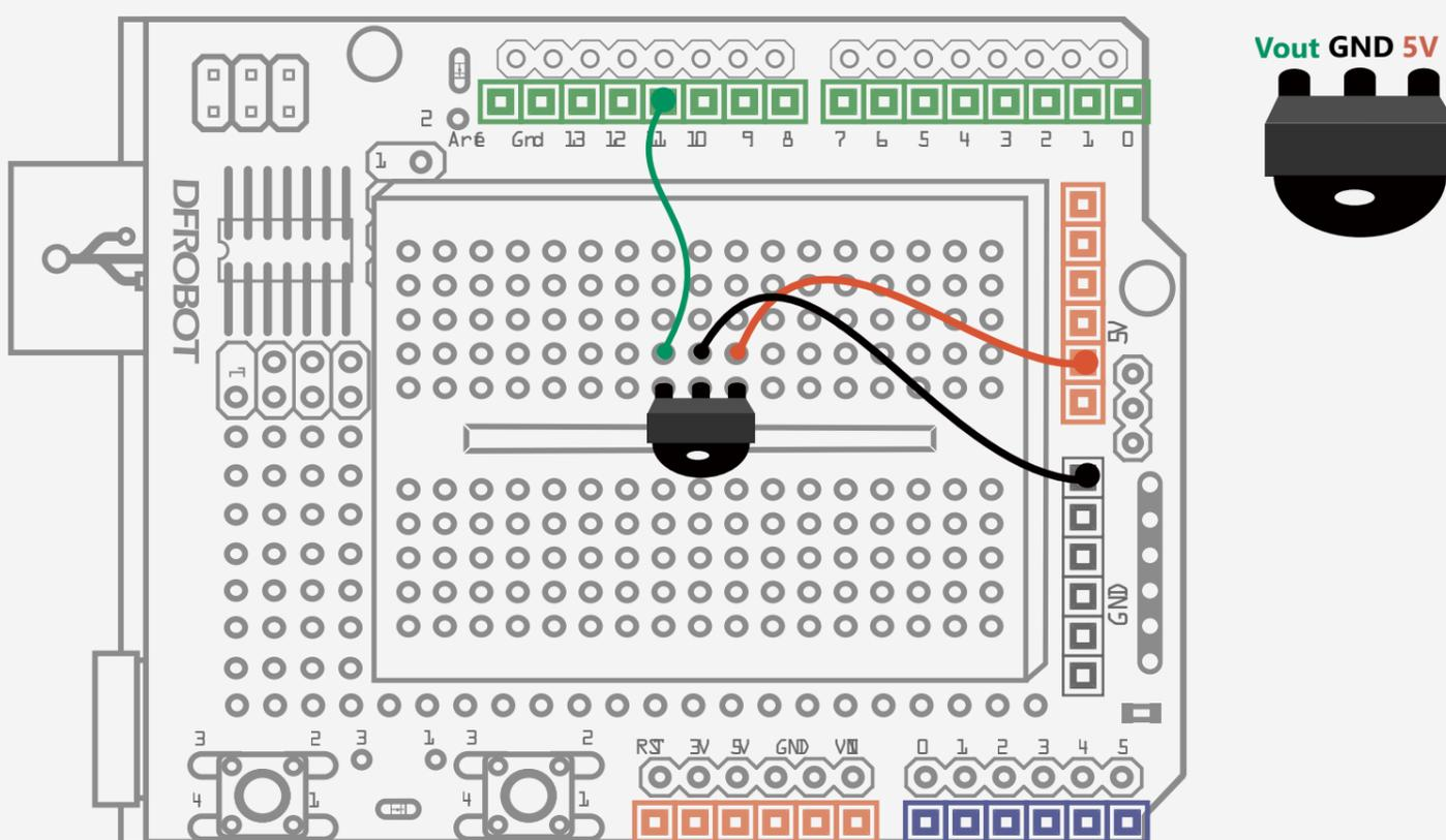
Fig. 14-1 IR Receiver Diagram
