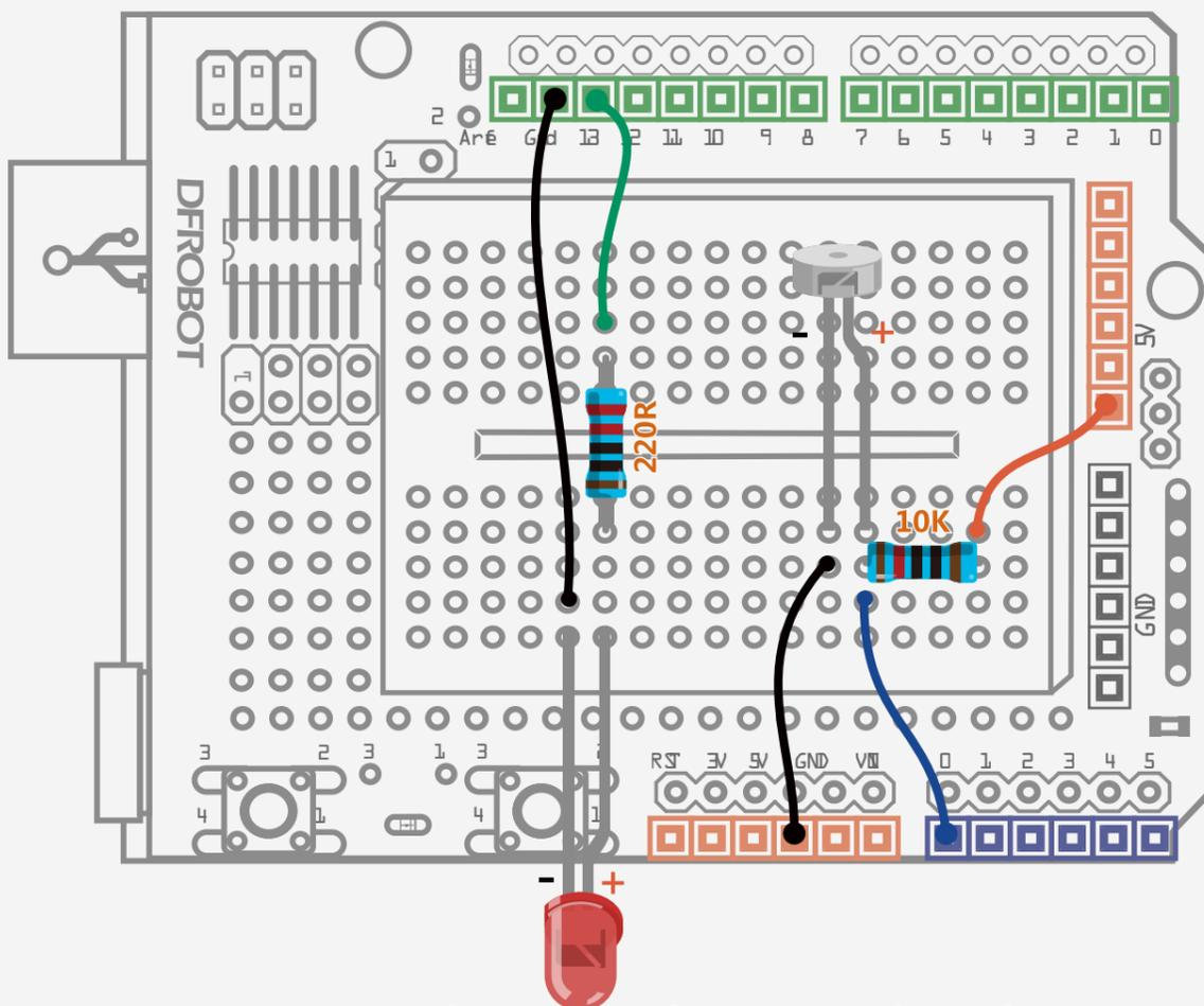
Diagram of the photo diode circuit
