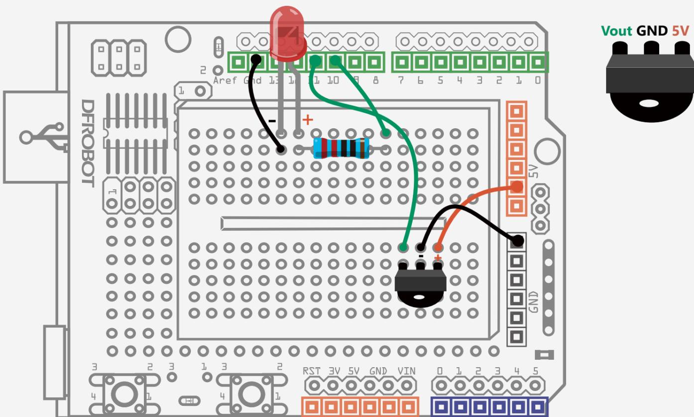
Fig. 14-2 IR Remote Controlled LED Circuit Diagram
