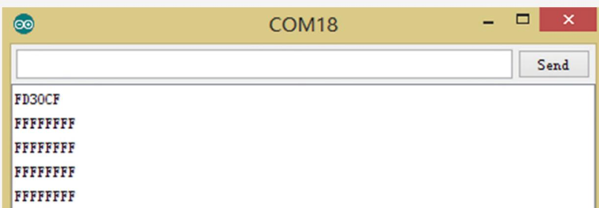
If it is received properly in the serial port, the code should be six digits starting with FD. If the controller does not send out the signal towards the infrared receiver, it might receive wrong code as we can see below.
