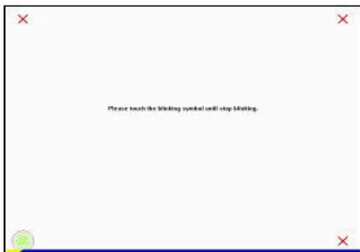
Touch the blinking symbol on the panel until it beeps or stops blinking.
