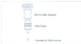
VGA connect via DVI to VGA adapter for DVI port product
