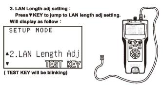
\* Connected the LAN Cable is known the length from MAIN connector to open .
