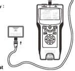
\* Press TEL KEY or TEST KEY start to test
