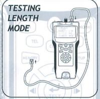
Testing from MAIN RJ45 Connector to open cable on other end.
