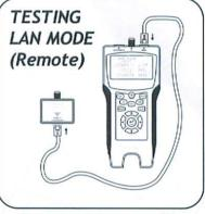
Testing From MAIN RJ45 Connector To REMOTE RJ45 Terminator Connector.
