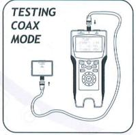
Testing From F Connector To REMOTE F Terminator Connector.
