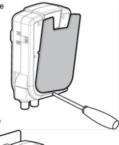
2. Remove the center screw from the faceplate of the wall outlet. Leave the faceplate in place.
