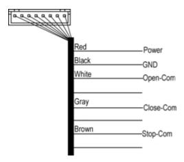
Once the harness is wired to the relay, plug it into the Curtain Signal Module. *Note that the connector is keyed and can only be inserted in one direction. Do not force the connectors together.*
