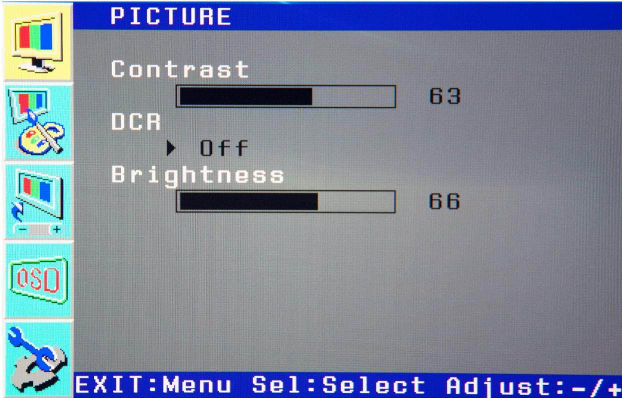
With the highlight in the top box on the left, press the **SELECT** button to enter the Picture submenu.
