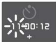
5. Use the **Video** and **Photo** buttons to increase or decrease the value of the blinking portion of the display. The **Video** button increases the value, while the **Photo** button decreases it.
