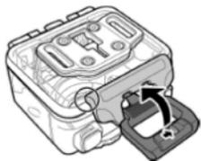
3. Swing the rear door open to reveal the empty camera housing.
