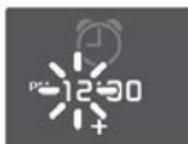
4. Use the **Left** and **Right** buttons to change which portion of the time display is blinking.
