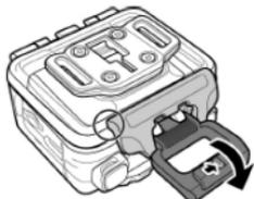
8. Press down on the front portion of the latch until it locks into place.
