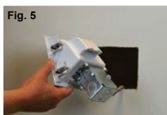
Figure 5: Use the four provided screws to secure the Steel Electrical Box and Receptacle to the mounting studs on the backside of the Recessed Low Voltage Mid-Side Plate.
