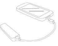
2. When your device is fully charged, unplug the charging cable from the Power Bank, and then from your mobile device. The Power Bank will remain on for about 15 seconds, and then will automatically turn off.
