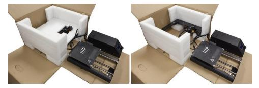
4. Carefully cut the zip tie that secures the **Extruder Assembly** to the **Tower Frame**.
