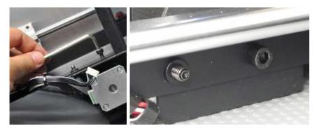
9. Use a carpenter's level to ensure that your flat surface is level. If it is not level, locate a level surface and place the printer on top of it. Next use the carpenter's level to check that the X-axis guide rods are level. If not, raise or lower either side by manually turning the Z-axis couplers on either side of the frame.
