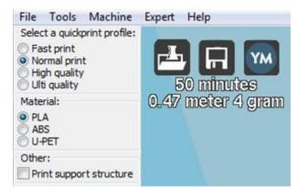
**Material** - Select one of three different material options, depending which type of filament you will be using. The printer ships with sample **PLA** filament, but you can also select **ABS** or **U-PET**, which is a newer filament material that combines the benefits of PLA and ABS.
