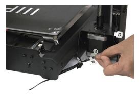
14. On the left side, insert the white connector labeled **C** into the white connector on the stepper motor, also labeled **C**.
