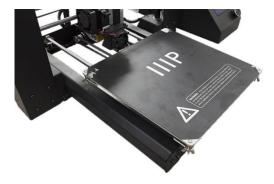
17. One by one, squeeze each corner of the built platform and tighten the knurled nut to compress the spring and reduce the distance between plates to the minimum.
