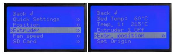
25. Insert the included MicroSD™ card into the slot on the side of the Power Supply, then select **SD Card > Mount Card**. Finally, select **SD Card > Print File**, select one of the sample 3D model files, then press the knob to start printing.
