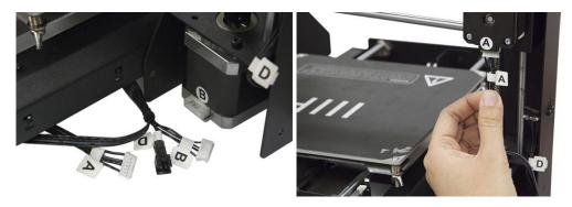
13. On the left side, insert the long cable connector labeled **B** into the motor connector, also labeled **B**.
