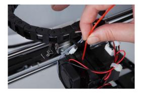
24. While holding the filament in place with one hand, select **Extruder > Extr. Position**. Push gently downward on the filament while turning the knob clockwise. You will feel the filament being pulled into the extruder. Continue until a few inches of filament material extrudes out of the nozzle. Carefully clean the extruded filament material off the print bed and nozzle.
