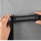
11. You can mount the **Filament Stand** and **Spool Holder** onto either the **Tower Frame** or the **Power Supply/Control Box**. Use two hex screws and the hex wrench to secure it to your desired location. If mounting it to the tower frame, ensure that the spool holder is mounted over the center of the tower frame.
