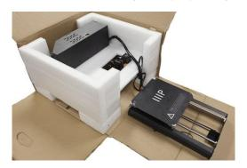
3. Remove the **Power Supply/Control Box**, place it next to the base, then remove the foam insert.
