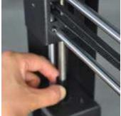
10. Remove one of the plastic nuts from the threaded end of the **Spool Holder**, but leave the second nut in place. Insert the threaded end of the spool holder through the **Filament Stand**, from the side opposite the base support. Thread the plastic nut onto the spool holder and tighten the plastic nuts on each side of the filament stand.
