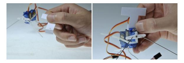
Use scissors to cut the sensor holder out of a plastic sheet, cardboard, or aluminum. You can even use a Dremel tool and cut it out of an old CD or DVD. Make sure the upper part is a minimum of 45mm wide to attach the infrared sensor. The base needs to be 10mm wide to attach the holder on the servo.
