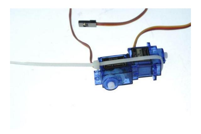
Wrap a big cable tie (4x200mm) around the two servos to secure them. Pull the cable tie very tight to strap the servos together. You may use pliers to give it the final pull.
