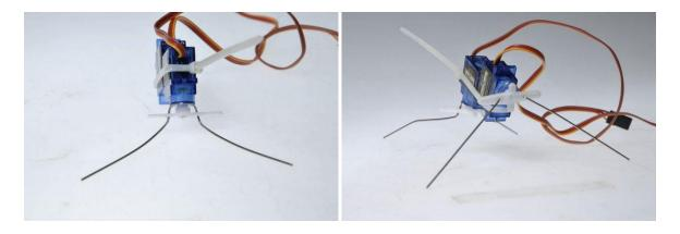
Attach the servo horns with the wire legs to the servo by fixing them with the small screw. For that step you should be familiar with Arduino and how to center a servo. Please center your servos first. If your servos are not centered, you can fix it later after switching the robot on for the first time. Bend the legs into a shape so that the robot is standing nice and stable.
