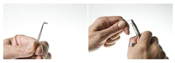
Bend the wire in a V shape as shown in the images above The tips of both wire ends should be 100mm apart. Don't worry about precision yet, you will have to bend them later in the right shape anyway.
