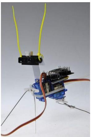
Use two sticky pads on each side of the battery. Then stick the battery on the bottom of the PCB and make sure it's aligned to the front. Remove the protective layer of the bottom side of the battery and stick the whole battery-board-assembly on the rear servo.
