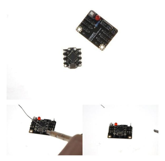
Now it's time to solder the Beetle controller onto the Beetle shield. First you have to put the beetle on the pins by paying attention to the right direction. The USB socked needs to face to the left side of the shield, the side where these two mounting holes are located.
