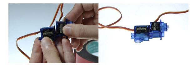
Stick both servos together by using double-sided foam tape. Front servo shaft in top and rear servo shaft on the backside. Make sure you align them properly so that they make a nice body for the robot.
