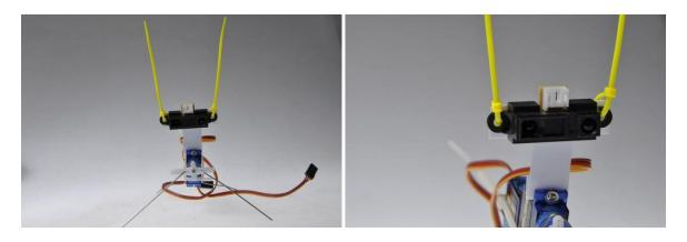
Make two holes for the infrared sensor by placing the sensor on the holder and mark the holes. Then make holes with with a 2mm diameter using scissors or another suitable tool. Fix the sensor with the white connector facing up on the holder by using two small cable ties. You may cut the cable ties but they are good to use as antennas or feelers. The sensor can also be attached using suitable bolts and nuts.
