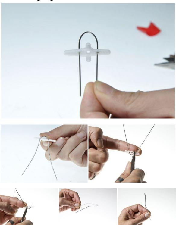
Put the two ends of the wire leg through the second hole from the center and then bend the two legs apart, as seen in the images above. Hold the wire leg and the servo horn with pliers and bend the wire down close to the servo horn.
