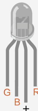
Fig. 5-5 Common Anode RGB Diagram
