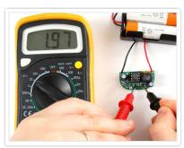
Next check between the rightmost pin and the second and third pin. They should both be at just about 2.0V
