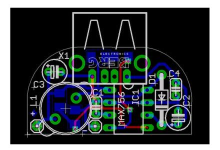
I actually do another etch test, to verify eveything one last time. Then I tile two boards together (cheaper) and generate gerbers.
