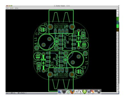
I always check the boards with <a href="www.freedfm.com">www.freedfm.com</a> (<a href="http://adafru.it/c4j">http://adafru.it/c4j</a>) before I ship them off to be made. I used 4pcb.com so it's the same company but even if you don't go with 4pcb.com as your PCB manufacturer, it's a neat service.
