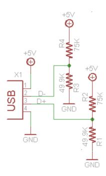
This time both voltages on the data lines are = 49.9K / (49.9K + 75K) \* 5.0V = 2.0V
