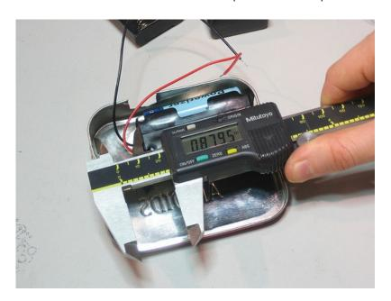
I also try out another battery holder I have, this gives me more space, 1.25"x0.85"...but the batteries go in sideways so one would have to remove the holder to change the batteries. I'd prefer that you can just take them out directly, so I don't go with this one (it also turns out I don't need that extra space).
