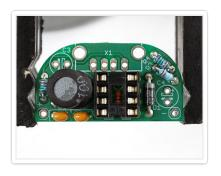
Next is the power inductor **L1**. This component is used by the DC/DC converter chip to store and convert power from low voltages to high. Inductors are just a coil of wire so they have no polarity and can be placed either way.
