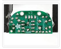
Solder in the two capacitors then clip the wires.
