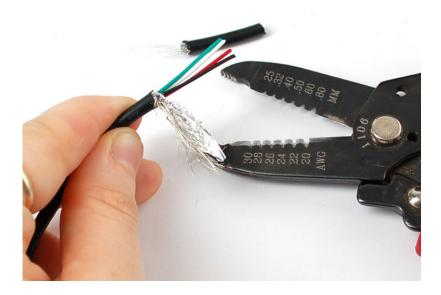
Shown above, the 4 wires. Red is power, black is ground, and the white and green wires are the data lines.
