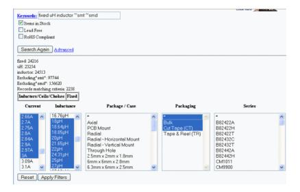
That filters it down to about a dozen choices. The SLF inductor is actually surface mount, and we're going to outright ignore the ones that cost more than \$2.50. Inductors for small electronics like this should cost around \$1-\$2, as a guideline. That leaves us with the DN7418-ND "INDUCTOR 27UH POWER AXIAL" and the 6000-220K-RC "INDUCTOR HI CURRENT RADIAL 22UH." Both of these look good, with about  $\sim 1.5$ A saturation current and 0.07 ohm DC resistance.
