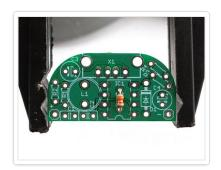
The first part we will place is the resistor **R5** - this is a small oval tan thing with two wires (leads) and color stripes. The stripes are orange orange red which indicates a 3.3K resistor. This resistor is used to improve the high current capability of the boost converter chip and is a new addition to the mintyboost. The resistor goes right in the middle, over the silkscreen text that says **R5**.
