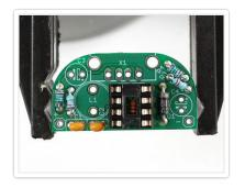
Next is the IC socket. This protects the chip and allows you to replace it if there are any problems. The socket goes *over* the 3.3K resistor but the resistor should not interfere as long as it was soldered in properly.
