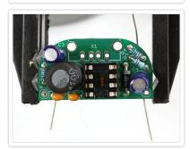
Next are the two electrolytic capacitors. These help smooth both the input and output voltages, to keep them stable during the up-conversion. They are used for low frequency noise, and are often paired with a ceramic capacitor.
