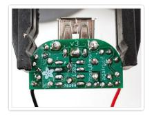
If you are having trouble getting the device to recognize the Mintyboost as a charger, it could be because it only wants 'USB spec' chargers. This is easy to do with the Mintyboost and always worth a shot as it will get most stuff up and running.
