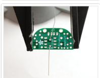
Bend the resistor into a staple and slip it onto the top of the Printed Circuit Board. Bend the little leads out so that you can flip over the PCB and the resistor will stay in place.
