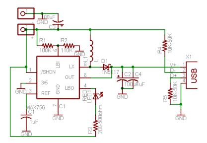
After a few months it became clear that some devices especially Apple music players, needed pullup/down resistors, so a new version that could fit 1 pullup and 1 pulldown was designed. This version still used the MAX756 (http://adafru.it/c3T).
