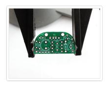
Place the PCB in a vise, and turn on the soldering iron. Make sure you have all the tools you'll need to assemble the kit (http://adafru.it/c3s).
