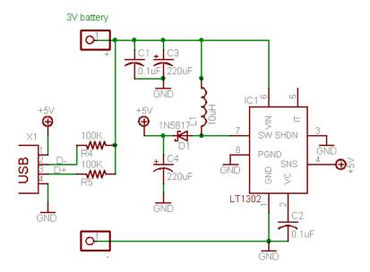
Smartphones started coming out and becoming popular, and devices with massive batteries, which meant that charging at 100mA was a no go. The mintyboost was then upgraded to the LT1302 (http://adafru.it/c3U), a more expensive chip but one with a nice 500mA output ability!
