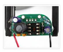
Next, solder in the 2xAA battery holder. The red wire goes to the hole marked + and the black wire goes to the hole marked -.
