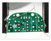
We will now finish up with the resistors. grab the last two left, these are  $49.9 \, \text{K} \, 1\%$  resistors and have Yellow White White Red Brown stripes. They go into the slots **R1** and **R3**.
