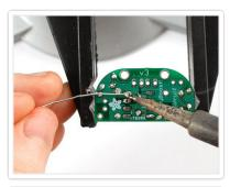
The socket has short legs so it can be annoying to keep in the right position. Hold it in place with one finger and 'tack solder' a corner.
