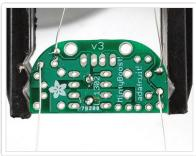
Solder the resistors as you did the 3.3K one, one point at a time, checking your work.
