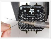
Solder in the capacitor's two legs just like you did with the resistor
