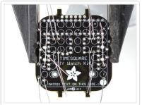
Solder in all the resistors, either one at a time or all 8 at once! Make sure you don't forget any solder points, though.
