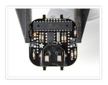
Next we'll place both the battery holder, and the timing crystal. The battery of course is how we power the watch, and this holder keeps it in place. The timing crystal is the "Quartz Crystal" in watches, that keeps time by resonating
