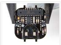
The battery holder will slip out if you flip over the board, so before flipping the board, solder one leg side from the top. The holder is a great heatsink so it may take a little longer than usual to solder in
