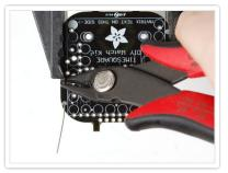
Once the soldering is complete, we can clean up by clipping the leads of the resistor. This keeps them from shorting to something else. Use diagonal or flush cutters to clip the wires right above where the solder joint ends.
