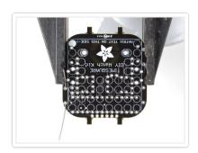
Bend the wire leads out so the resistor sits flat against the PCB. Then you can flip it over and it wont fall out!
