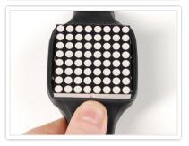
Place the clear back first into the band so it's at the bottom. Then stretch the band and scootch the assembly in, pulling the rubber to fit around!
