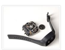
Get the remaining parts out of the kit - a 20mm coin battery, silicone band and optional clear plastic back
