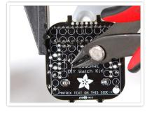
Flip it over and solder in the other battery pin, then go back and do the first one.
