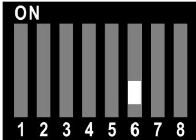
To enable the Power/Status LED, set DIP switch #6 to ON:
