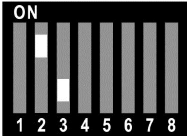
To force the RGB sync signals positive, set DIP switch #2 to ON and DIP switch #3 to ON:
