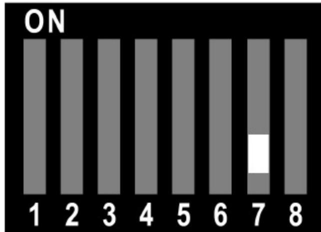
To enable 1080p support for Port 2B, set DIP switch #7 to ON:
