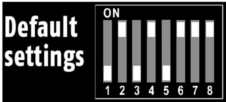
For convenience, the default factory settings and DIP switch features are printed on the back of the HDfury3:
