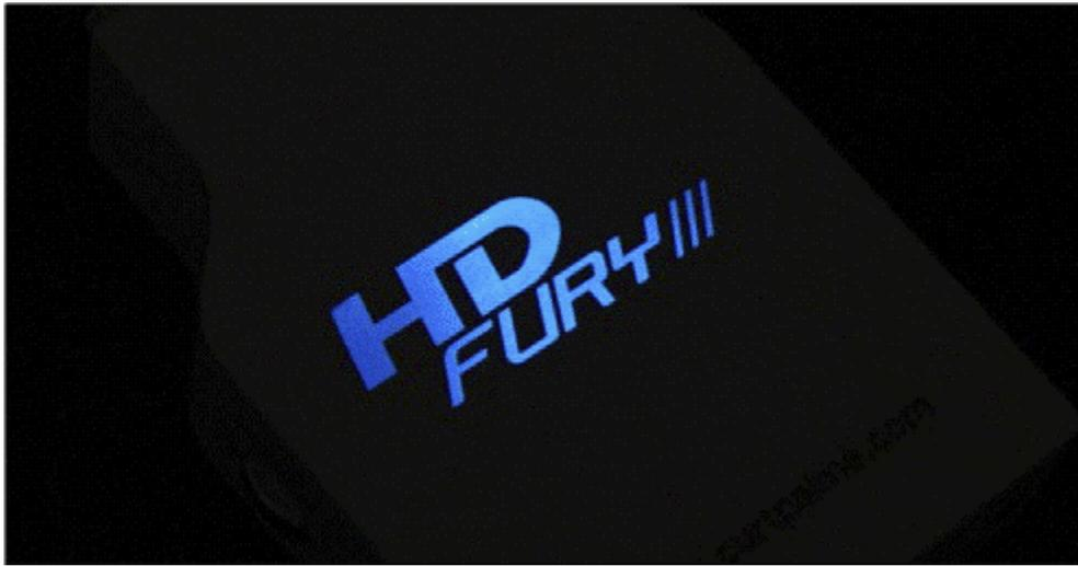
The HDfury3 logo will glow blue when in use. When the HDfury3 first receives an HDMI signal the logo will quickly turn on, then off, and then on permanently to indicate that the HDCP handshake has been completed.
