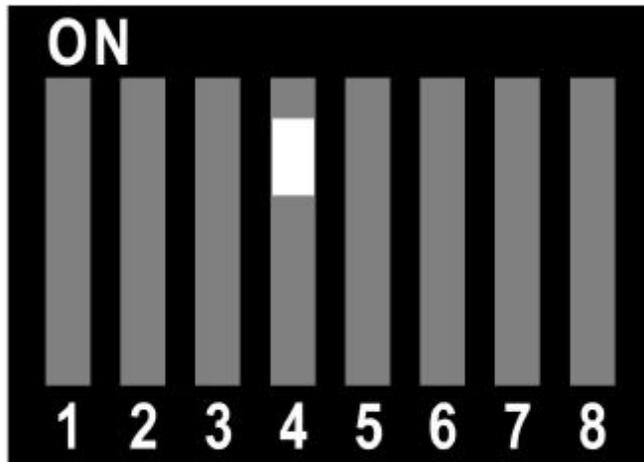
To disable this feature and use normal colour depth (16-235), set DIP switch #4 to OFF:
