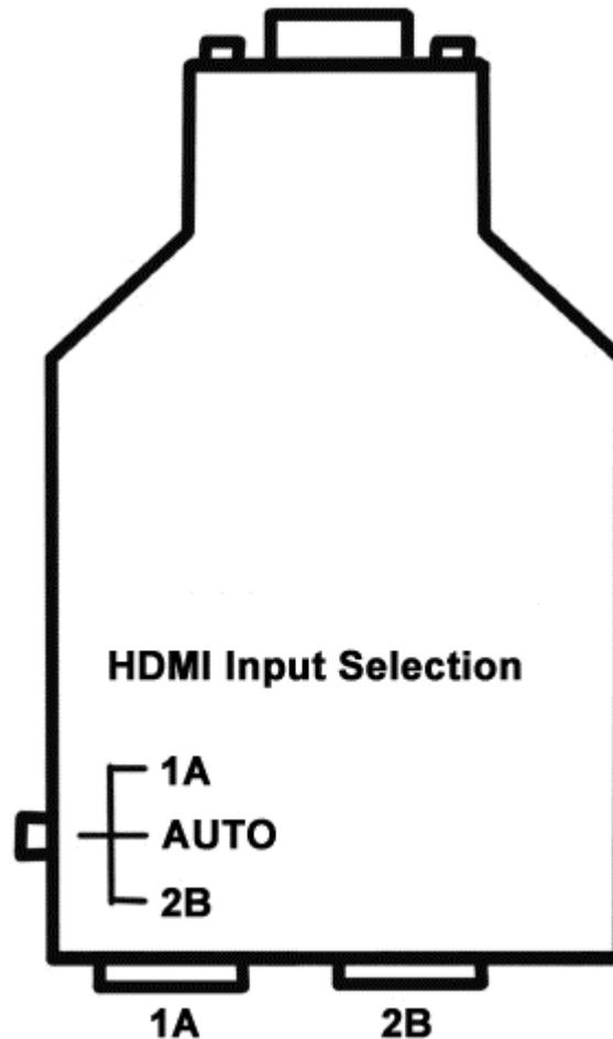
The HDfury3 has two HDMI-inputs. The “1A / AUTO / 2B” switch may be used to select the active HDMI input as follows:
