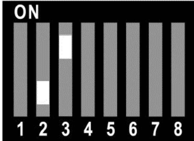
To invert the RGB sync signals, set DIP switch #2 to OFF and DIP switch #3 to OFF:
