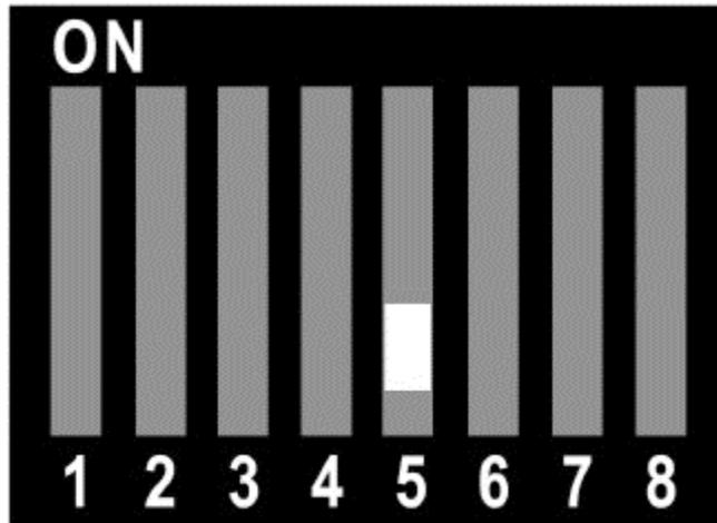
To enable the RGB Shift button, set DIP switch #5 to ON:
