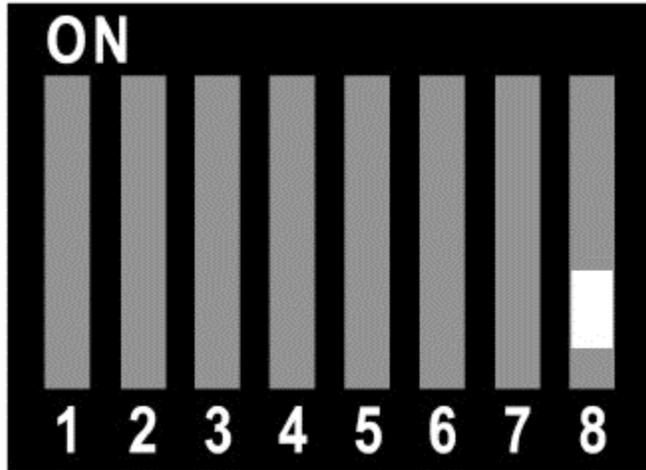
To enable 1080p support for Port 1A, set DIP switch #8 to ON:
