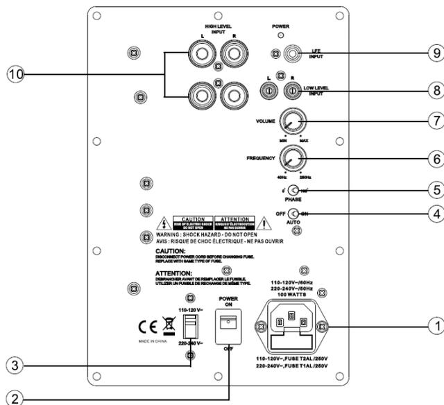
5. **PHASE:** Sets the subwoofer to be in-phase or 180° out-of-phase with the signal being sent to the satellite and center channel speakers. See the *SETUP* section below for details on how to use this control.
