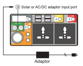
plug the other end into a nearby AC power outlet. The Charging Input LED Indicator (2) will glow Red and the LCD Display (1) will blink the current charge level.
