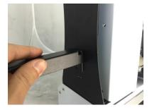
paper can be slid between the nozzle and the platform without binding. When the extruder head is moved or when the paper is moved under it, there should be a slight amount of resistance, but the paper should not be dragged with the extruder when it is moved.
