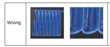
The nozzle is too close to the platform. This can result in damage to the nozzle and build platform.
