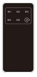
IN1、IN2、IN3、IN4、IN5: Press these buttons will force switch the input port and the LED will indicate the corresponding input source.
