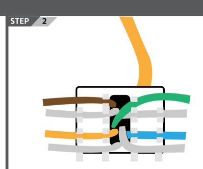
Follow the labelled colors on the modular covera and set each wire into the proper position to ensure the ground wiring connects properly.
