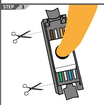
Place the assembled modular cover into the module and cut the wires evenly to fit.
