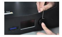
18. Manually turn the Z-axis screw clockwise to raise the print bed.
