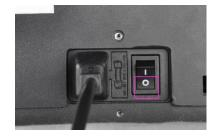
22. Insert the C13 end of the included AC power cord into the C14 panel connector
