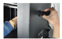
21. Ensure that the printer is powered off (O side of the power switch is depressed).
