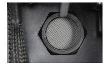
20. With one hand hold the nut in place. With the other hand insert the spool holder into the large hole on the back, then turn clockwise and thread it into the nut. Tighten, but do not over tighten.
