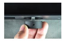
17. Using the 1.5mm hex wrench, tighten the locking screw to secure the control knob in place. Ensure that there is a small amount of clearance between the knob and the printer frame so the knob can be freely moved.
