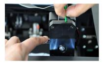
6. Turn the control knob clockwise until your filament starts to extrude out of the nozzle. Note that the initial material coming out of the nozzle may not be the same color as your filament. This is because factory testing of this printer may have left some
