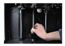
19. Insert the plastic spool holder nut into the hex shaped indent inside the printer. Position the wrench mark on the nut toward the 2 o'clock position.
