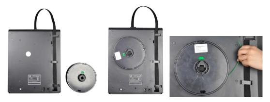
4. Select the **Move material** option. Wait for the nozzle temperature to reach the target value (200°C).
