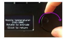
residual filament in the nozzle. Keep turning the control knob until the correct color material starts to extrude. Press the control knob to continue.
