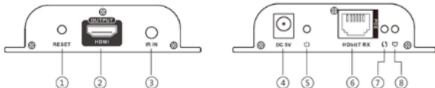
1. **Reset:** Button for restarting the receiver.
