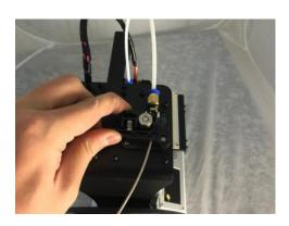
19. Using the included plastic scraper, clean the extruded filament from the nozzle and build platform.
