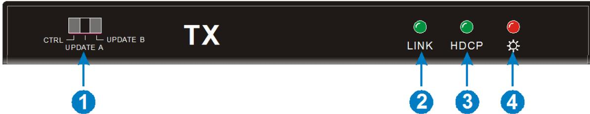
1. **RS232 MODE Switch:** Selects the RS232 mode. The **CTRL** position is the normal operating mode where RS232 data is passed back and forth with the receiver. The two **UPDATE** positions are for updating the transmitter's firmware using one of two methods. See the *FIRMWARE UPDATE* section for details.
