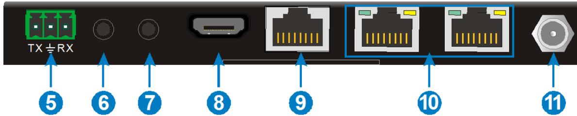
5. **RS232 Connector:** Connector for the included 3-pin to DB9 RS232 cable.
