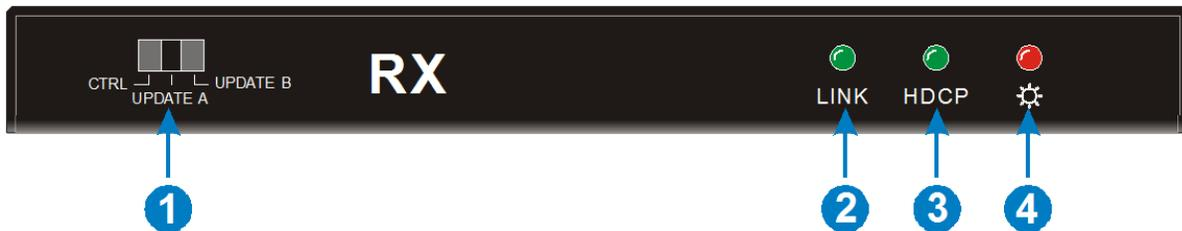
1. **RS232 MODE Switch:** Selects the RS232 mode. The **CTRL** position is the normal operating mode where RS232 data is passed back and forth with the transmitter. The two **UPDATE** positions are for updating the receiver's firmware using one of two methods. See the *FIRMWARE UPDATE* section for details.
