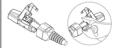
Use pliers to clamp the wiring cap closed until it completely snaps in to complete the connection.
