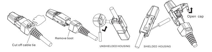
Cut off the cable tie, and remove the boot. Using a flat screw driver, gently pry open the plug cover one end at a time.
