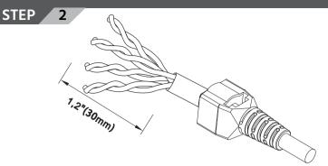
Insert the cable into the strain relief boot, then strip off 30mm of the cable jacket and fold back the braided and drain wires.
