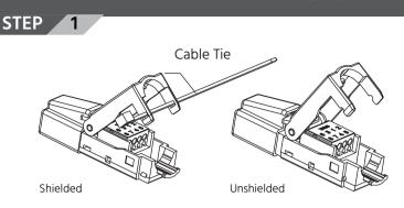
Remove the cable tie before installation.
