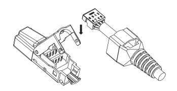
Place the wiring cap onto the plug
