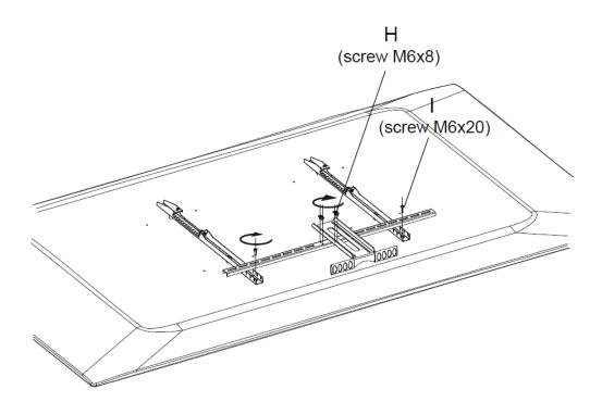
11. Using two people, lift the television and hang the hooks on the front panel. Then use a Philips screwdriver to tighten the two locking screws on each bracket, which secures the brackets to the front panel.
