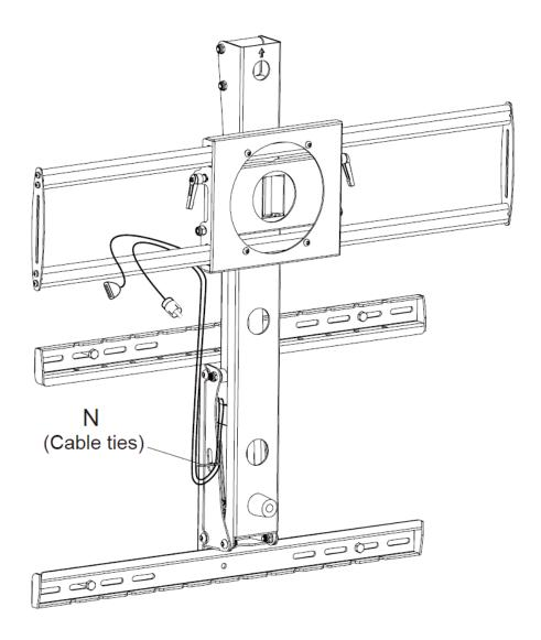
9. Place a towel or blanket on a flat surface, then place your television face down on it. Attach the hooks (BB) to the back of the television using the appropriate screws, washers, and/or spacers. The proper combinations to use are the Philips pan head screws (B) and washer 1 (F), Philips pan head screw (C) and washer 1 (F) and spacer (G), Philips pan head screw (E) only, or Philips pan head screw (E) and spacer (G).
