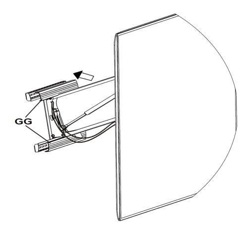
13. Adjust the spring pressure to balance the weight of the display so that it can be easily moved and will maintain its position using either a ratchet wrench or the hexagon wrench (O) provided.
