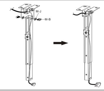
Attach the adjustable rod to the ceiling plate with four screws and four washers.
