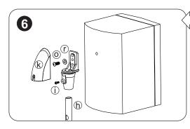
BOSE ACOUSTIMASS LOUDS PEAKERS Attach universal bracket(h) to pole using screw (i) Feed cable down pole as shown in fig 3a or 3b. Attach loudspeaker to bracKet using screw (o) and washers (r).
