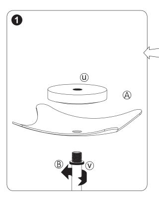
Insert assembled tube (B) into base (A) and screw
