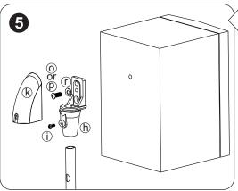
FOR LOUDSPEAKERS WITH THREADED HOLE Secure universal bracket(h)to upright using screw(i). The speaker cable should be Connected to the speaker and threaded through the upright as shown in fig 3a or 3b. The speaker should be fixed to bracket (h) Using washer(r)and either screw(o) or (p) depending on speaker type, Fit cover cap (k) if required.
