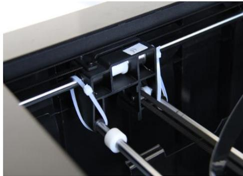
7. Remove the top cover from inside the printer.
