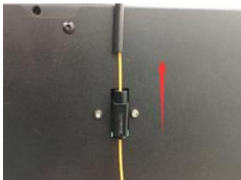
4. Insert the filament guide tube into the filament detection mechanism.
