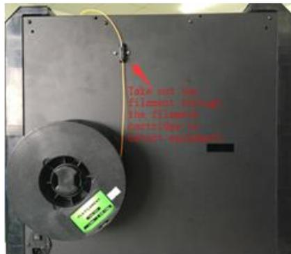
3. Feed the filament through the filament guide tube.
