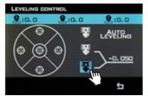
5. Adjust the height of the nozzle until it pinches the paper, checking each time whether the paper can be moved or not. Once the paper cannot be moved, return to the main menu and touch to home the printer.
