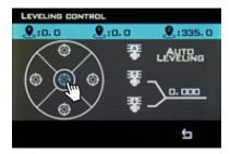
4. Touch For to adjust the height of the nozzle up or down.
