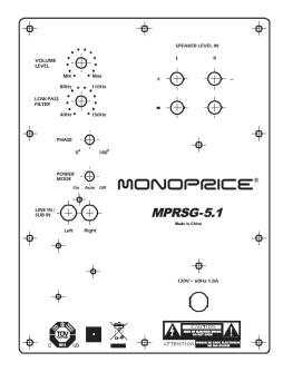
subwoofer is therefore used to match the audio output level of the satellite and center channel speakers so that they blend into one smooth, continuous sound. In general, unless your musical material is particularly bass heavy or light, once you have set the volume on the subwoofer you shouldn't need to adjust it again.
