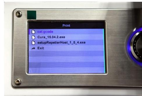
21. After the first layer has been laid down, use the control wheel to **Pause** or **Cancel** the printing operation. Examine the layer and compare the printed material with the images in the table below. If the result is wrong, turn off the printer and re-adjust the platform height as indicated. Clean off the printed material using the included plastic scraper, then print the model print again. Keep repeating this process until the result is correct.
