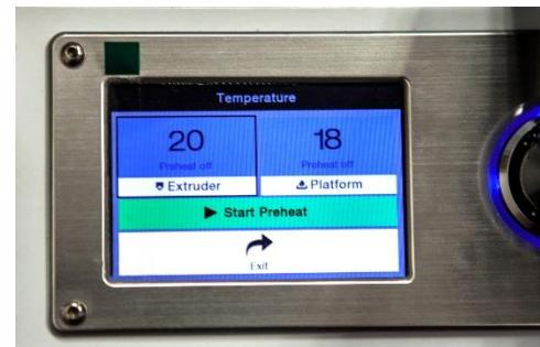
13. If the button under the Extruder and Platform reads Start Preheat, use the control wheel to highlight the **Start Preheat** entry, then press it to start preheating the extruder and build platform. The button will change to read Stop Preheat and the Extruder and Platform buttons will read the actual temperatures.
