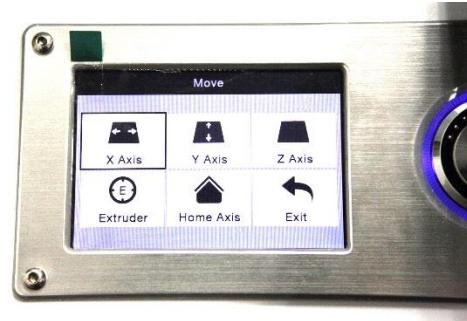
paper can be slid between the nozzle and the platform without binding. When the extruder head is moved or when the paper is moved under it, there should be a slight amount of resistance, but the paper should not be dragged with the extruder when it is moved.
