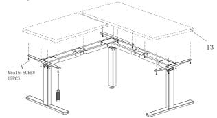
6 Mount the control box (8) under desktop(13) with screws (A). Use the screws (A) to install the controller panel(12) under the desktop. If using two separate table boards, connect and support them with the table connection hardware (10).
