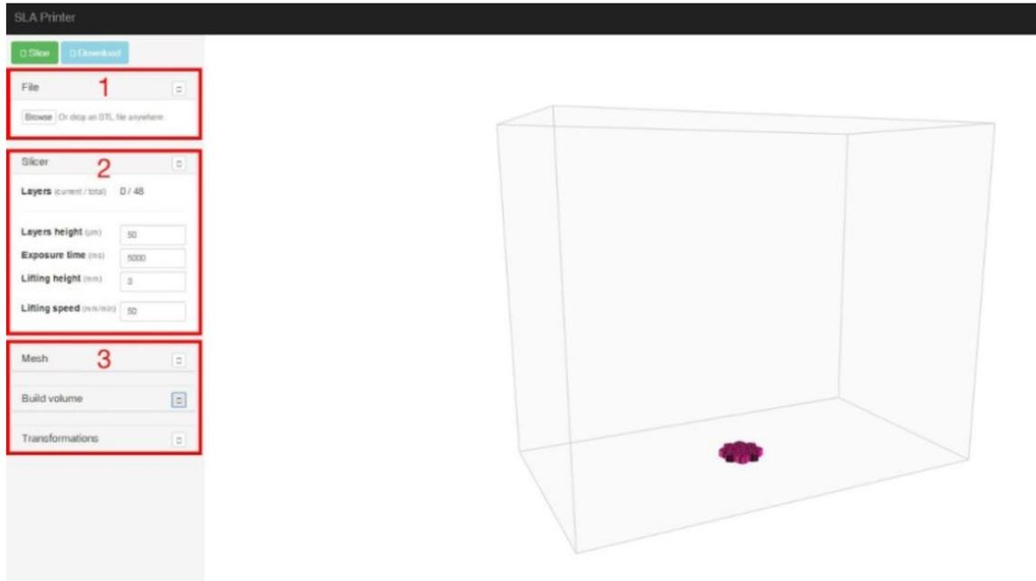
1. Upload an STL 3D model file by dragging and dropping the file onto the Web Slicer screen.
