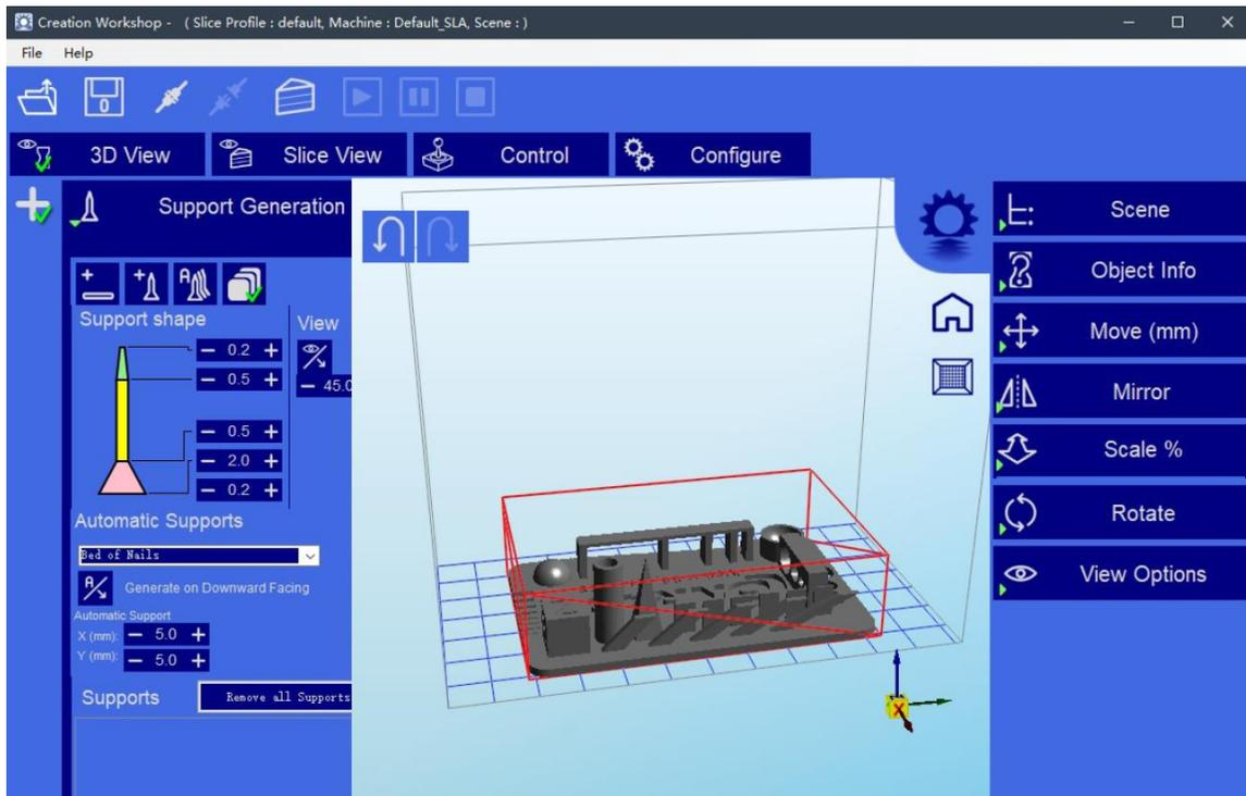
After the model has been loaded, you can add supports, as needed.
