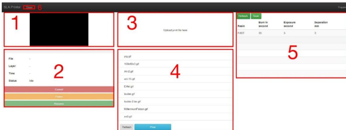
1. Displays an image of the current layer being printed.
