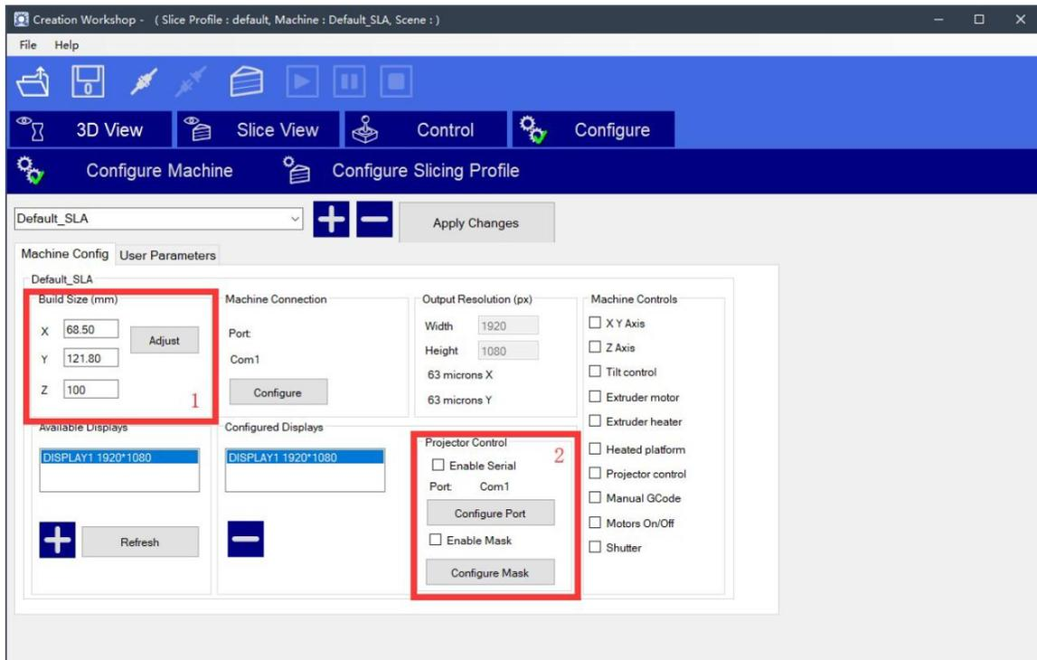
If the print size is different from the actual size, you can change the display size. Correct the print size by adjusting the XY values in the **Build Size (mm)** section. Click **Apply Changes** to save your settings.
