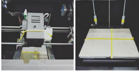
3. Use the included 2mm Allen wrench and the included spanner to remove the fixed support on the Z-axis.
