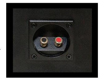
The ideal connection is through the two line level RCA jacks, while spring loaded terminals can be used to accept speaker level inputs, if line level is not possible. The spring-loaded terminals can accept bare speaker wire (up to 9 AWG) or pin plugs.
