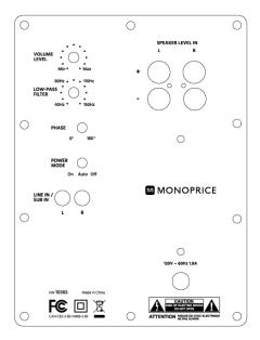
Low-Pass Filter: The low-pass filter determines how well the bass from the subwoofer blends with the mids and highs from the satellite and center channel speakers. Because the satellite and center channel speakers have a frequency response that starts at about 110Hz, we want the subwoofer to handle all frequencies up to 110Hz. A good starting point is to set the low-pass filter at 110Hz and then adjust it slightly up or down according to how it sounds.
