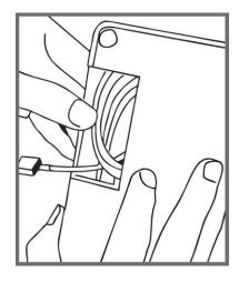
7. Plug the USB Type-A connector on the Apple Watch cable into the **USB** port inside the base.
