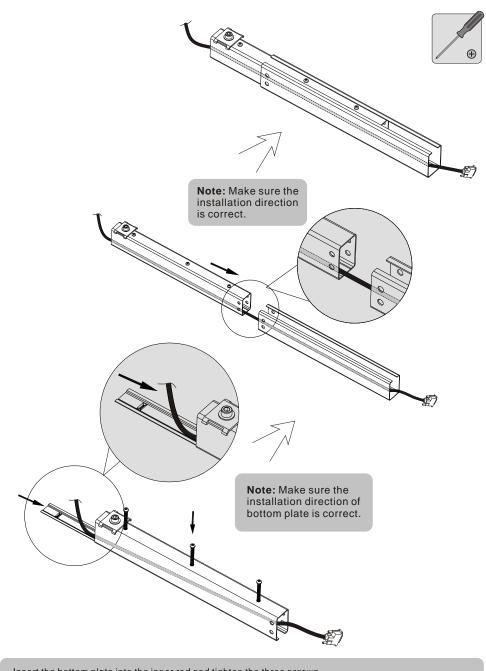
Insert the bottom plate into the inner rod and tighten the three screws.
