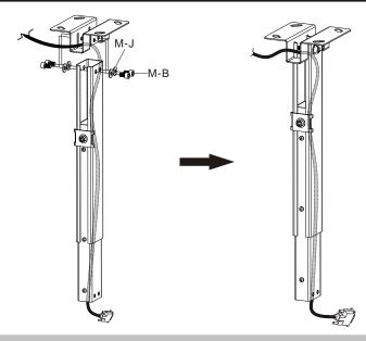
Attach the adjustable rod to the ceiling plate with four screws and four washers.
