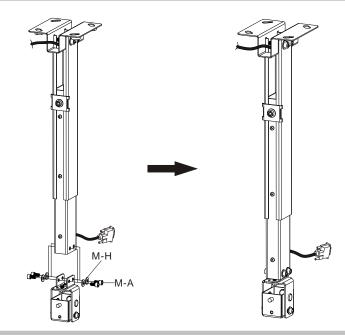
Insert the pivot bracket into the end of inner rod and secure with four screws and four washers.
