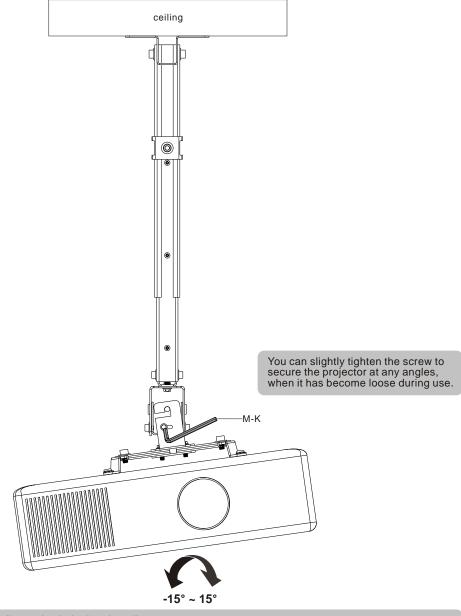
Adjust to the desired angle or tilt.
