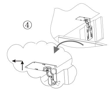
4. Attach the bracket to the ceiling.
