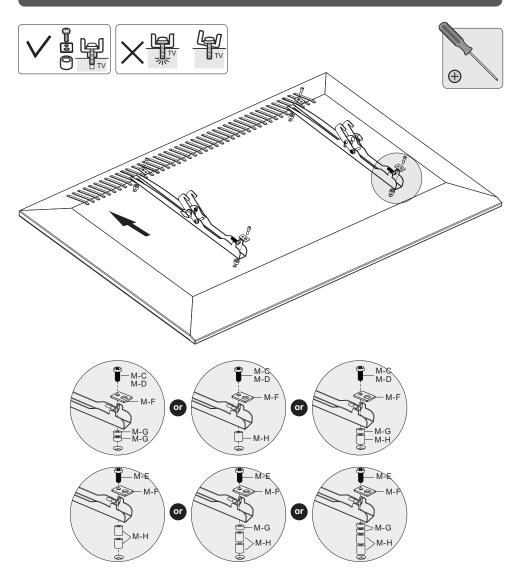
Note: Choose the appropriate screws, washers and spacers (if necessary) according to the type of screen. Position the adapter brackets as close as possible to the center of the TV.
