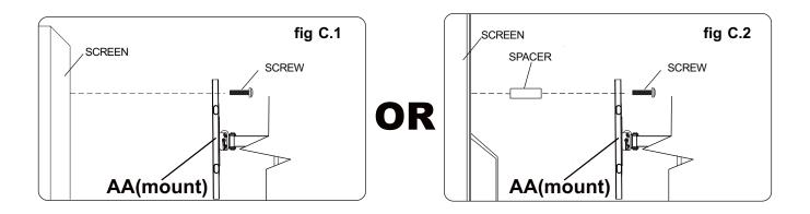
Select the small,medium,large or extra large screws from the baffled .Fastener pack then attach screen brackets(AA) to screen following figure C.1 or C.2 on page 7.
