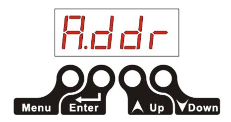
**MENU:** Press the MENU button to cycle through the DMX512, Dimmer, and Strobe modes. After setting a DMX512, Dimmer, or Strobe value, press the MENU button to accept the setting.
