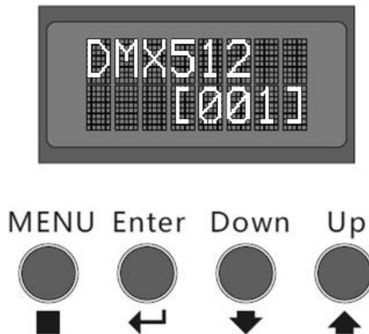
**MENU:** Press the **MENU** button to cycle through the DMX512, Dimmer (R, G, B, and W), Strobe, Fade, and Auto modes. After setting a value, press the **MENU** button to accept the setting.
