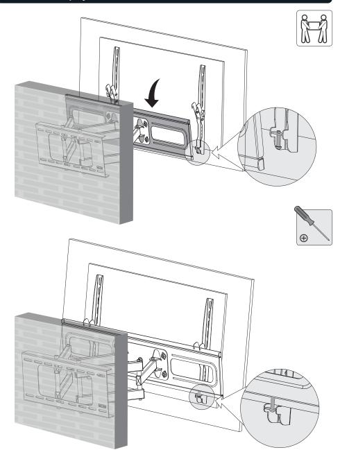
Tighten the bottom bolts by using a proper phillips screwdriver to secure the adapter brackets to the wall mount.
