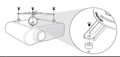
Place the Bottom Spacers in between the Extension Brackets and the Projector, and align the mounting.
