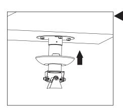
After mount is installed, slide cover bezel up and snap in place.
