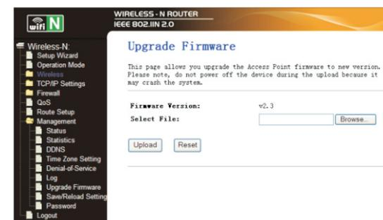
After a firmware upgrade file is selected, click 'Upload' button, and the router will start firmware upgrade procedure automatically. The procedure may take several minutes, please be patient.
